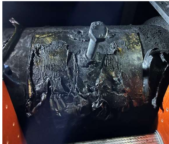
Left- Figure 8: Vent pipe section found on the deck of the boiler. Right- Figure 9: The removed section fits perfectly into the cutout section of the vent pipe. Both images taken on January 11, 2024, by U.S. Coast Guard.
