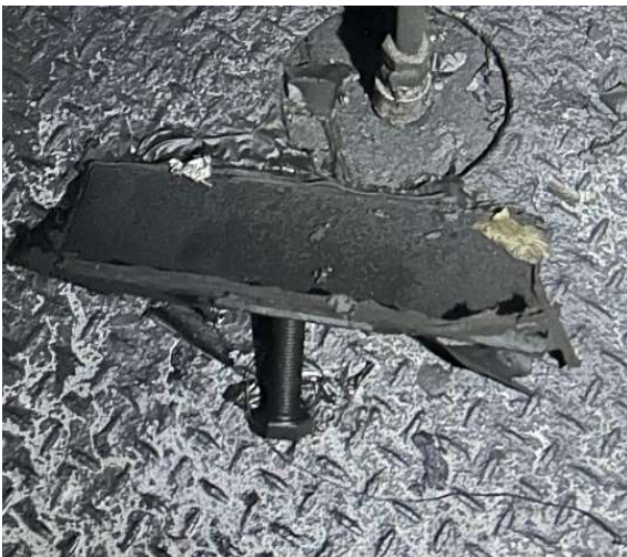
Left- Figure 8: Vent pipe section found on the deck of the boiler. Right- Figure 9: The removed section fits perfectly into the cutout section of the vent pipe. Both images taken on January 11, 2024, by U.S. Coast Guard.
