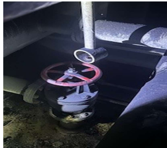
Left- Figure 3- Starboard double bottom diesel oil storage tank valve with attached reach rod. Right- Figure 4- Port double bottom diesel oil storage tank with reach rod hanging down but not attached. Images taken on January 13, 2024, by U.S. Coast Guard.
