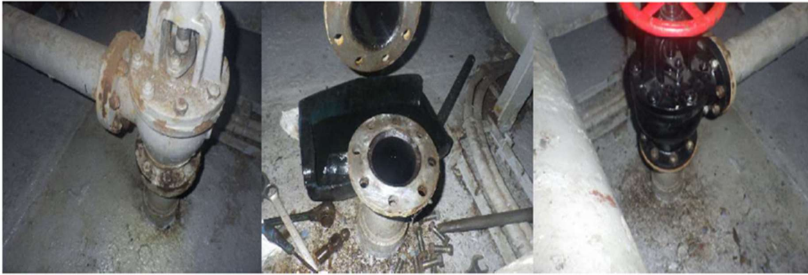
Figure 2: Images of the port double bottom diesel oil tank valve replacement from the 20-26 Nov-2023 Weekly Engine Jobs. Provided by Danaos Shipping Co. Ltd.
