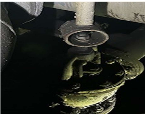
Left- Figure 3- Starboard double bottom diesel oil storage tank valve with attached reach rod. Right- Figure 4- Port double bottom diesel oil storage tank with reach rod hanging down but not attached. Images taken on January 13, 2024, by U.S. Coast Guard.
