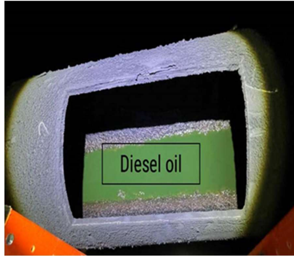
Left- Figure 6: Horizontal vent pipe section with cut out. Right- Figure 7: Diesel oil inside the vent pipe. Both images taken on January 11, 2024, by U.S. Coast Guard.
